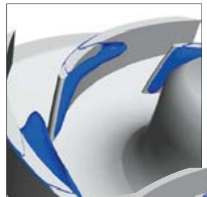
Below: CFX assists EMP in preventing cavitation problems. The blue areas in these pictures are isosurfaces that show where the static pressure of the water is below the vapor pressure, leading to cavitation. The pictures are different views of the same impeller.
