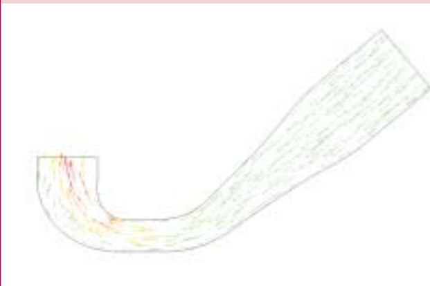
Velocity vectors on a 2-D slice plane of the inflow tube allow engineers to visualize the flow field through the pump inlet.
