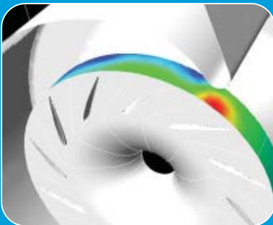
The distribution of static pressures at the fan rotor exit with the fan mounted inside a volute, which distributes the fan flow.
